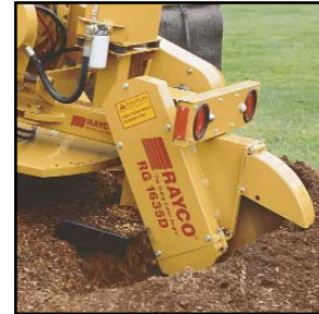
This compact machine makes a 71 inch wide cut.
