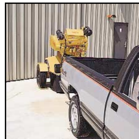
This high performance, tow-behind stump cutter is narrower than a standard pickup truck.
