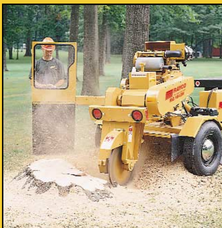
This high performance compact cuts 78 inches wide, 27 inches high, 24 inches deep, and it pulls back a full 60 inches.
