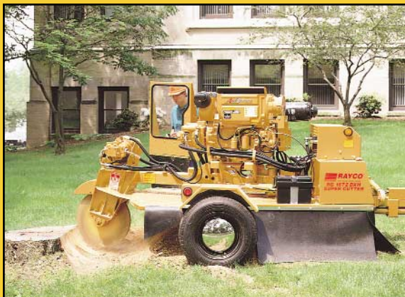
The RG 1672DXH's engine is mounted level on the chassis so it does not move with the cutter wheel.
