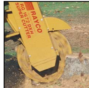
The variable speed, hydrostatic drive system can drive the cutter wheel from 0 to 1,150 rpm.
