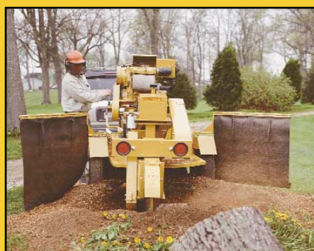
The RG 1635D can turn a 36 inch diameter stump into mulch in minutes.
