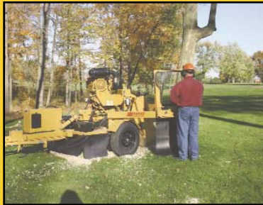
An electronically welded, steel chassis supports this compact stump cutter.
