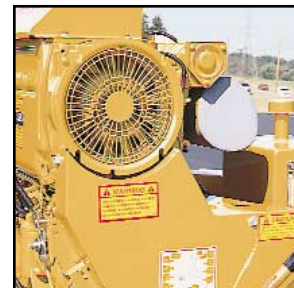
The RG 1660M is powered by a 60 HP Duetz turbo diesel.
