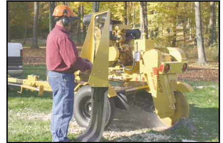
A swing-away control console provides a protected view of the cutting action.
