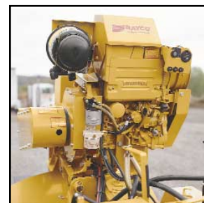
The RG 1635D is powered by an air-cooled, 31 HP Deutz diesel.
