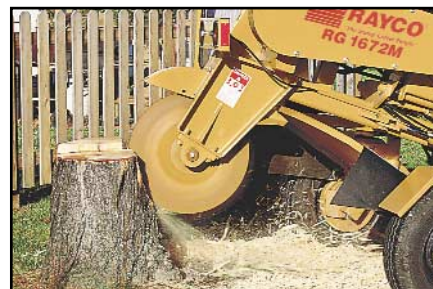
The RG 1672M will cut 29 inches high, 25 inches deep, and 81 inches wide without repositioning.
